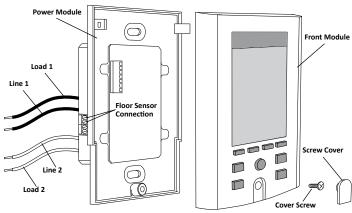
Match and connect the two wires marked "LINE1(L)" and "LINE2(N)" to the house power supply wires using the wire nuts provided. Gently tug on the wires to make sure they are secure, otherwise a wire could come loose and cause failure. For added security, overwrap the connections with electrical tape.
